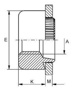
Female thread A = M2,5Height K = 3.0Outer diameter E = 6.0 Plate thickness = 1.7 to 1.9
